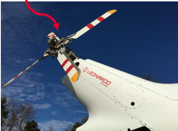
Air-cooled tail motor unit
