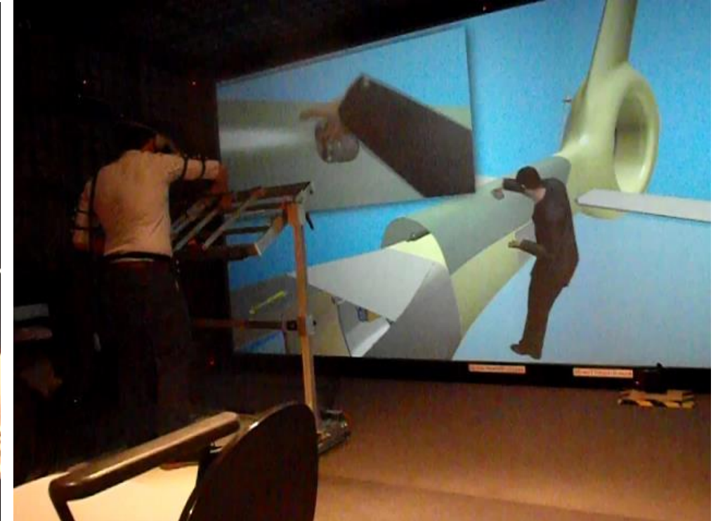
Inspection of rear transmission shaft
